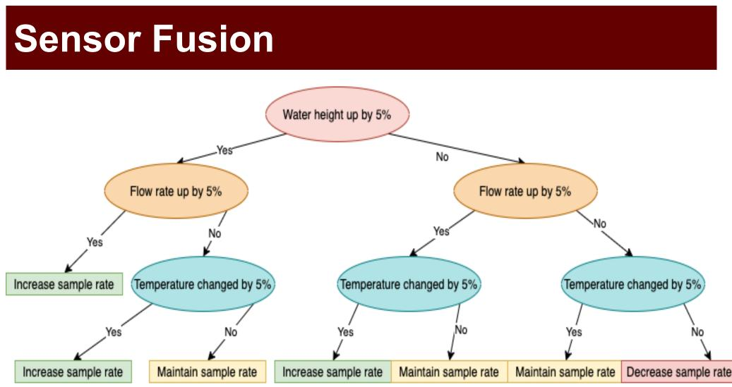
Device makes adaptation based on local sensor data • **Results:** increase, decrease or maintain the sample rate
